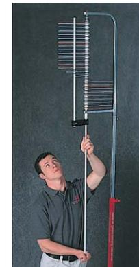
**4 Reset tool** aligns dislodged vanes for a clean target.
